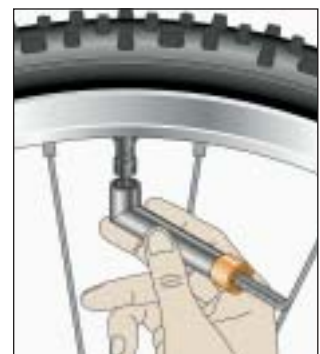
Inflation pressure checking with AIRMAX pressure gauge
