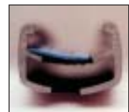
The rim tape is too narrow and does not secure the rim well.
